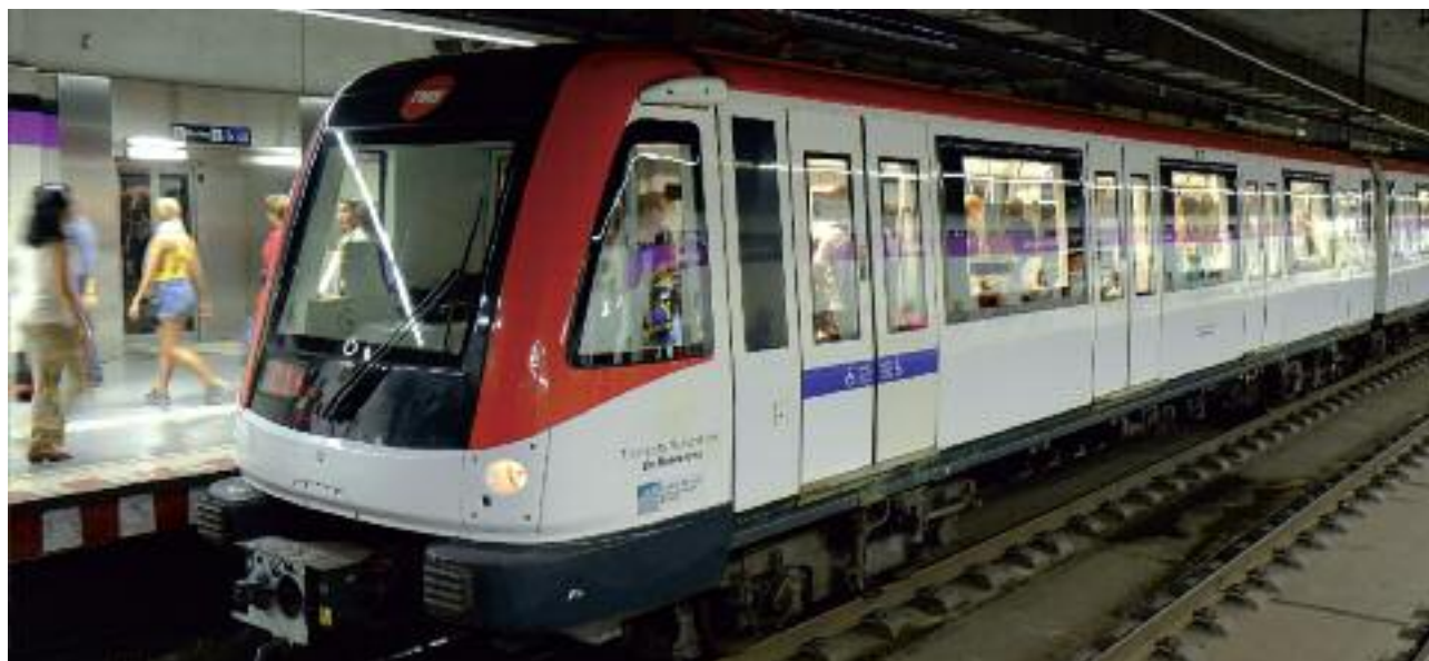
Series 9000 train, manufactured by Alstom, at Sagrada Família station on line 2. These were the first engines prepared to circulate without a driver, although drivers do operate on this line.
